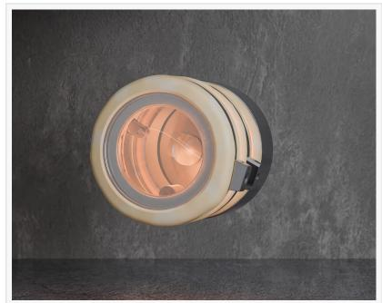
NS Nanotech's ShortWaveLight 215 Emitter integrates a nitride semiconductor that emits far-UVC solid-state light at 215 nanometers for photonic disinfection applications
