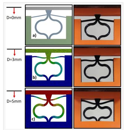
Comparison of the behavior of unit cell obtained from numerical and experimental results under different vertical displacements. Credit: Journal of Scientific Reports (2024). DOI: DOI: 10.1038/s41598-024-70126-x
