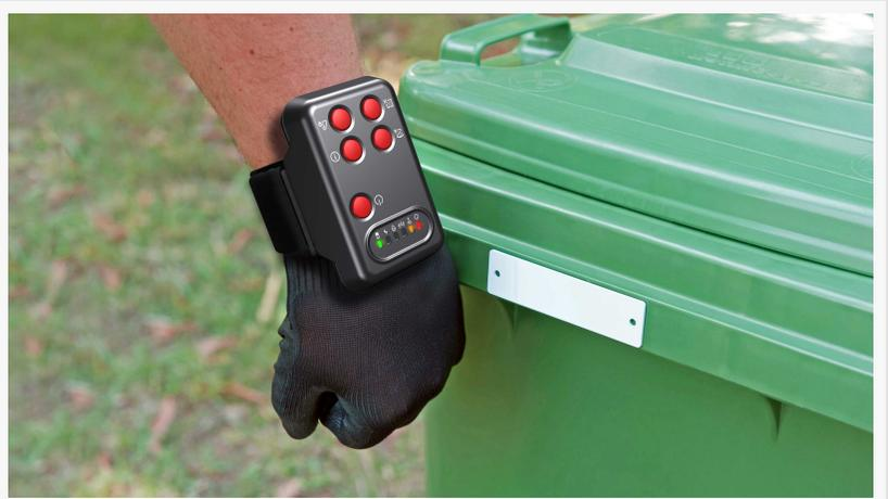
Discovery Mobile 3.0 wearable RFID reader reads RFID tag on waste bin
