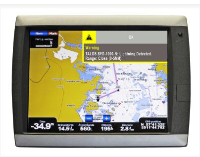
SFD-1000-N2K with marine navigation instrument and lightning warning displayed on the multifunction display screen with industry standard Parameter Group Numbers (PGNs).
