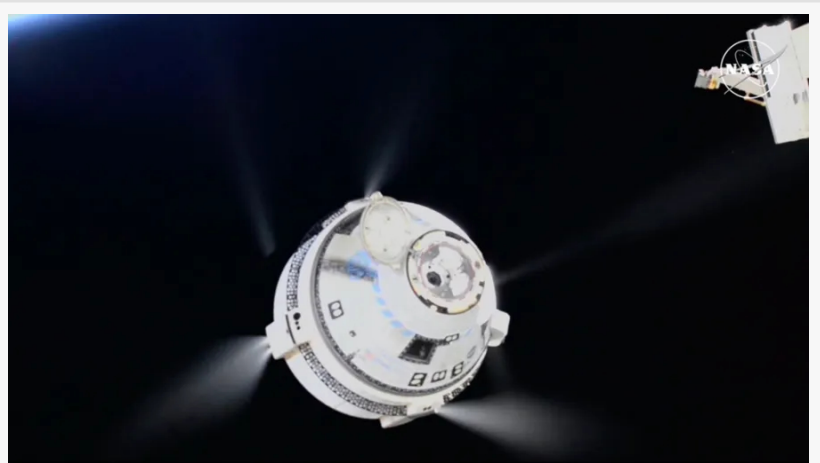
Starliner firing maneuvering thrusters as it departs the International Space Station. Credit: NASA
