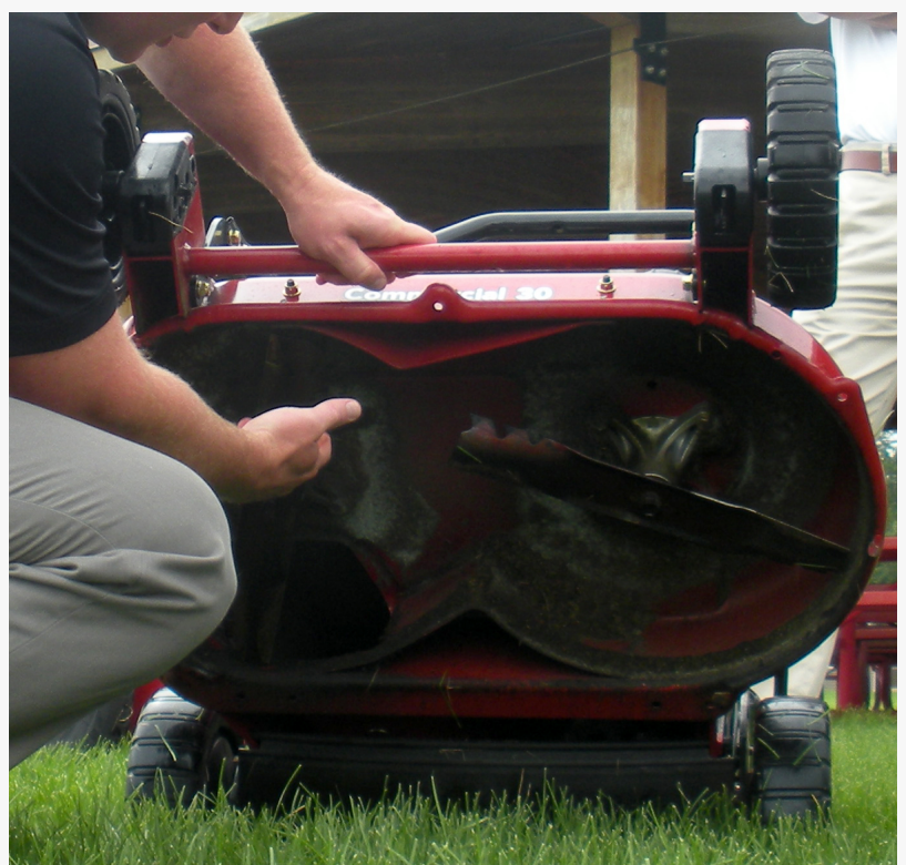
Most consumer walk-behind mowers have one or two blades to sharpen.
