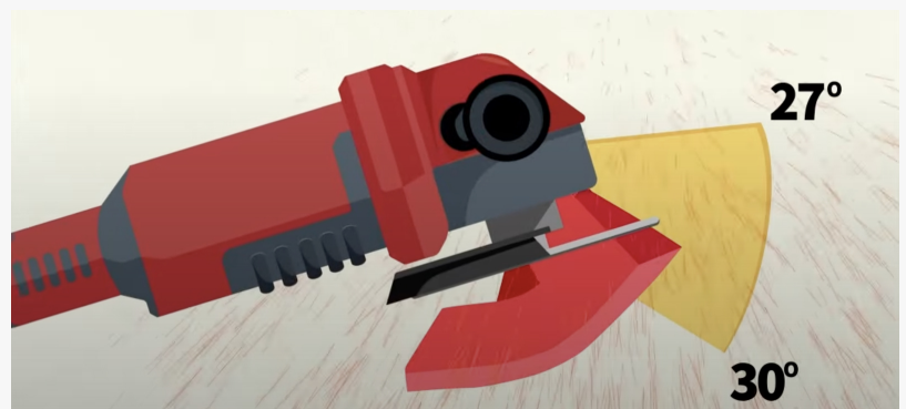
Sharpen blades at a 27- to 30-degree angle.
