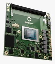
new COM Express Compact modules with AMD Ryzen Embedded 8000 Series for high-performance AI applications at the edge
