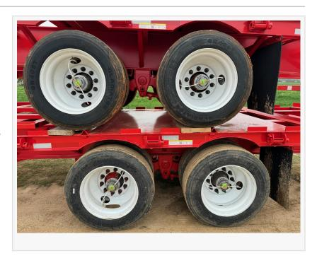
The P.S.I. (Pressure Systems International) Tire Inflation System brings a transformative solution to the challenges associated with tire pressure maintenance during poultry transport. By automatically monitoring and maintaining proper air pressure in trailer tires, the system ensures
