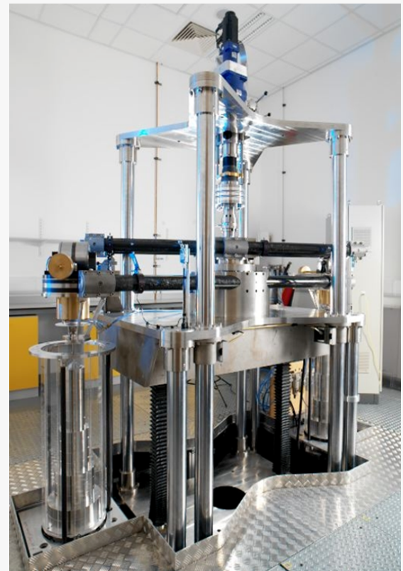
Morehouse Instrument Company's National Torque Standard.
