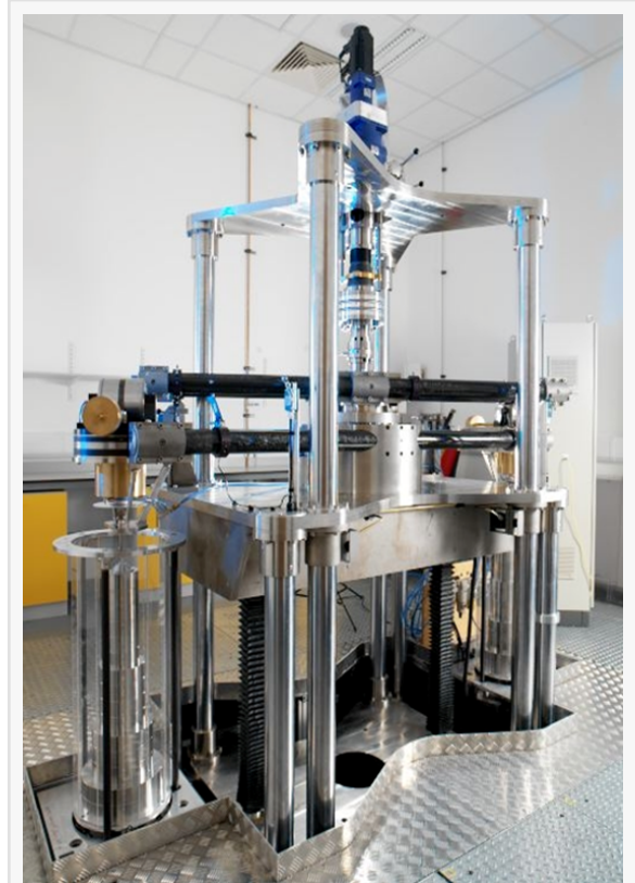
Morehouse Instrument Company's National Torque Standard.
