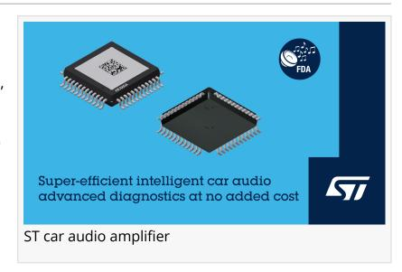
With its feedback-before-filter topology and 2MHz nominal PWM frequency, the HFA80A lets designers optimize the output filter for the targeted performance and achieve a compact outline with small component values. Spread-spectrum operation simplifies meeting the mandatory CISPR 25 specification, with no additional EMC-specific filtering required.
