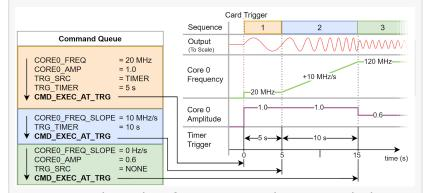
In DDS-mode, only a few commands are needed to, for example, generate a sine wave (orange block), accelerate the frequency (blue block) and lower the amplitude (green block).
