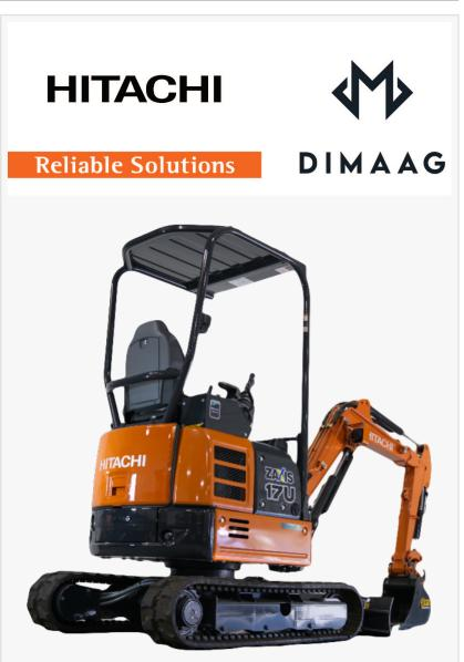
1.7-ton class electric excavator exhibited by Dimaag at CES2024
