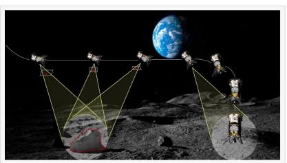
Artist rendition of LITPHAM used by a small class Lunar lander during its descent phases. In low illumination conditions, LITPHAM shines LED light while generating Digital Elevation Maps (DEMs) via Structure from Motion (SfM) to identify and avoid hazards during landing
