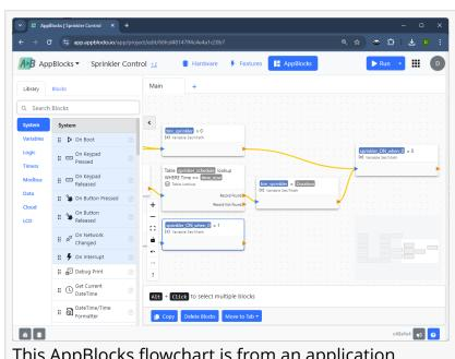
This AppBlocks flowchart is from an application designed to control a water sprinkler
