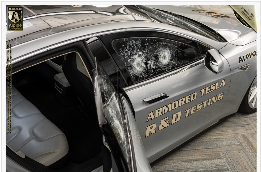
After the shooting the Alpine Armoring Armored Tesla S's passenger side shows that the glass was not penetrated by the test fire.
