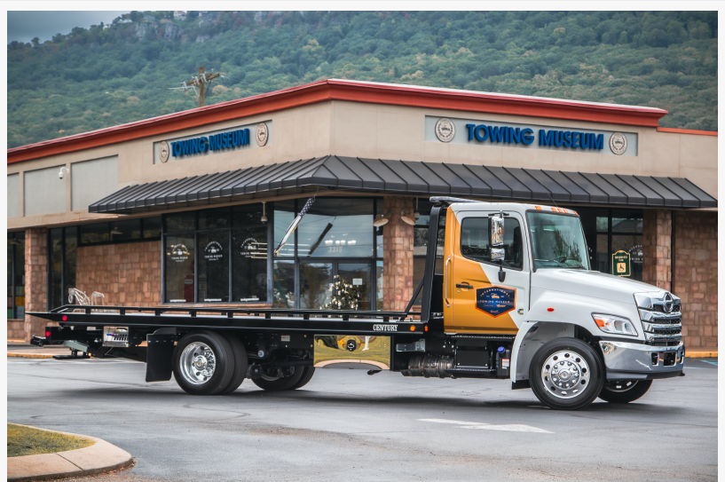
The winning tow truck is a Hino L6 Series truck with a Century 12 Series LCG™ bed by Miller Industries.
