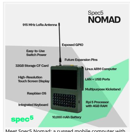
Meet Spec5 Nomad: a rugged mobile computer with touchscreen, keyboard, powerful ARM processor, multi-radio capabilities, and expansion options. Ready for any mission!
