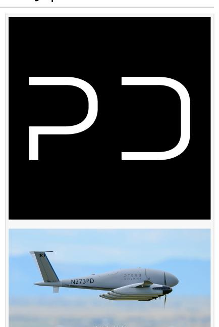
wing aircraft with superior VTOL performance in an efficient, highly automated platform. The aircraft folds its wings to transition seamlessly between vertical and winged horizontal flight,
