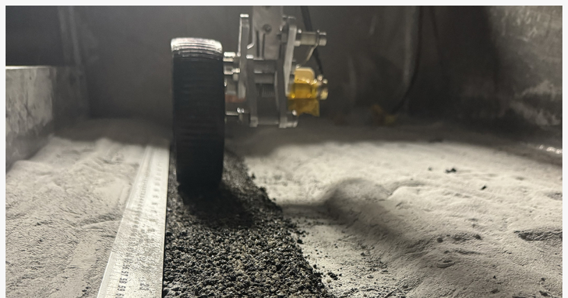
The SpaceFactory-MTU team successfully paved a lunar "road" in space-like conditions, driving 720 meters over the trackway.
