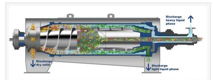
The centrifugal force generated enables the Sorticanter® to separate different types of plastic from each other. This enables operators to achieve the highest possible purity of plastics.
