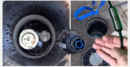
Electro Scan has developed probes that can be used by British Framework contractors to test leaks on customer properties, in pipes 25mm-50mm (1 -2 inches) diameter pipes and confirm lead pipes.
