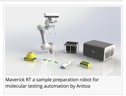
preparation cobot relies on computer vision instead of rigid position-actuation to achieve precise motion control required to handle liquid dispensing and pick-and-place of consumables such as qPCR test tubes.
