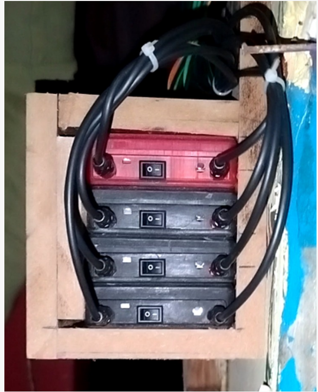
KC12V uses Series-Parallel Switching Circuit
