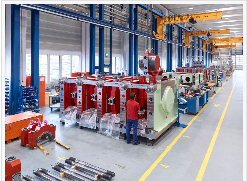
Hyper Compressor Assembly at Burckhardt Compression
