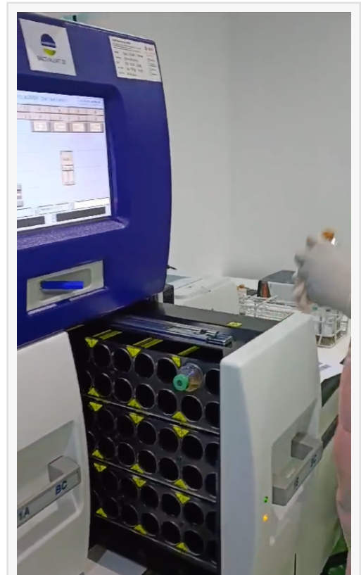
Sterility testing using the BacT/Alert 3D microbial detection system
