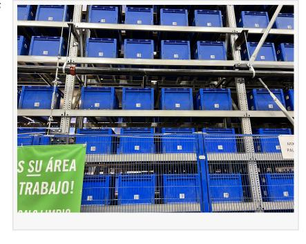
and an advanced, two-level product storage configuration using an automated automatic storage and retrieval system (ASRS).
