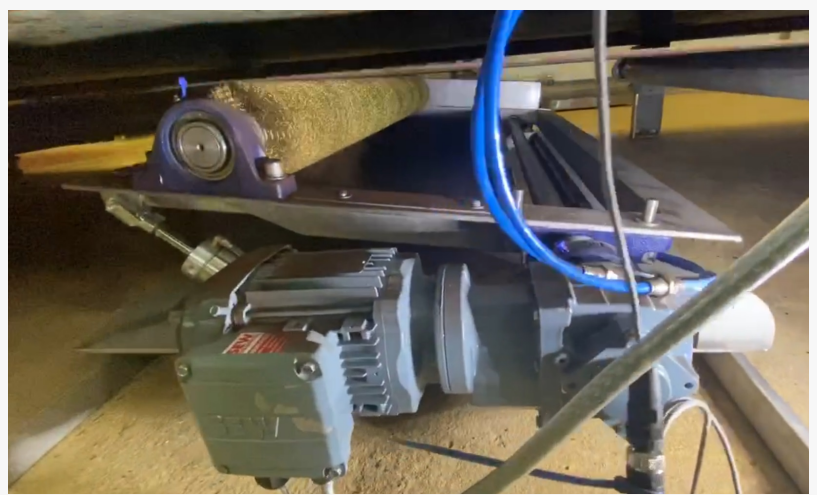
One of Continuous Process Solutions' innovative cleaning brushes in operation on a baking belt.
