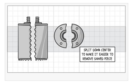
cuts and removes holes within wood. As woodworking tools continue to advance, users are consistently looking for new and specialized tools that save time and effort. The Split Hole Saw Bit fits perfectly within this niche market and would significantly enhance any manufacturer's product line.
