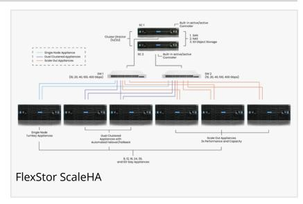
ScaleHA™ - a cloud-scale data center infrastructure configuration for StoneFly's Veeam Ready airgapped and immutable backup and DR solution (DR365V).
