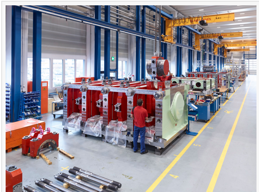
Hyper Compressor Assembly at Burckhardt Compression
