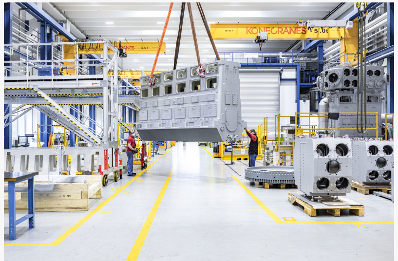
LABY Compressor in workshop
