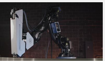
SpaceFactory plans to assemble ASTRA, a robotic 3D printer, at its new Huntsville facility. Designed to print large structures autonomously using recycled and locally sourced materials, ASTRA offers a flexible solution for point-of-need manufacturing.
