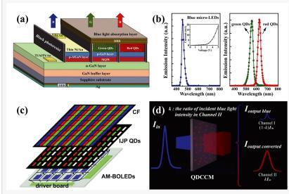
(a) Schematic configuration of the monolithic full color Micro-LED and (b) the EL spectra of the GaN-based blue micro-LEDs, the emission spectrum of the green and red QDs. (c) A schematic illustration of the architecture for the color conversion OLED disp
