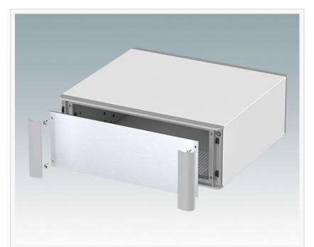
Anodized aluminum front panels are recessed in the TECHNOMET front bezel – protecting the controls and displays. All fixings are hidden by snap-on trims.
