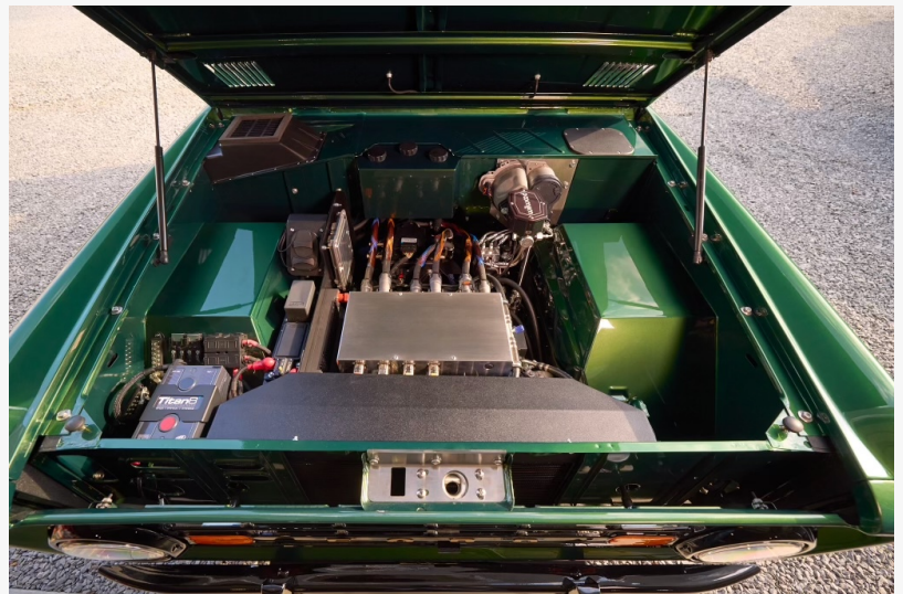
A detailed view of the advanced electric powertrain under the hood of Kincer Chassis' 1977 Ford Bronco, highlighting modern EV components.
