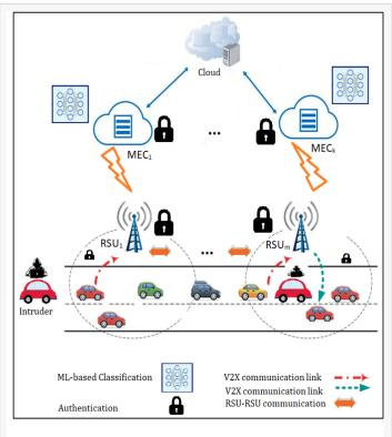
Fig. 1. Architecture of a secured distributed edge intelligence for IoV Architecture of a secured distributed edge intelligence for IoV.
