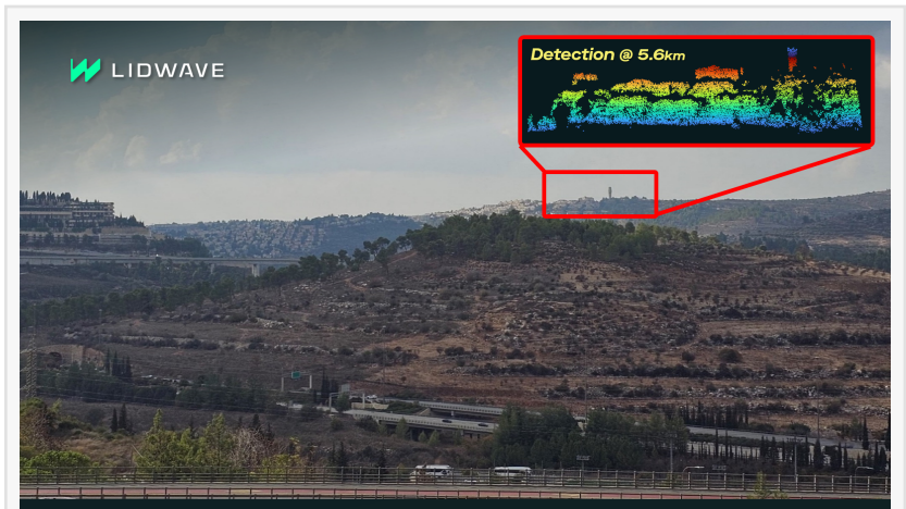
High-resolution (0.005X0.005 deg) zoom-in view to an object located 5.6 km away
