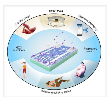
Igzo nanofibre-based sensors are integrated with a flexible circuit to create a sensory face mask, thus featuring wireless and real-time monitoring capabilities
