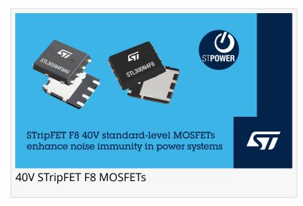
The industrial-grade STL300N4F8 and automotive-grade STL305N4F8AG MOSFETs have a drain current rating above 300A and maximum RDS(on) of  $1m\Omega$ , permitting outstanding efficiency in high-power applications. Enhancing dynamic performance, the total gate charge of 65nC (typical) with low device capacitances (Ciss, Crss) ensure minimal losses at high switching frequency. The MOSFET body diode assists efficiency and reliability with low forward voltage and fast reverse recovery.
