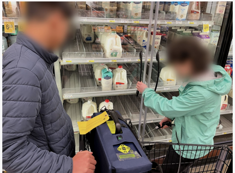
Detecting leaks with the Gasmeter in a grocery store aisle
