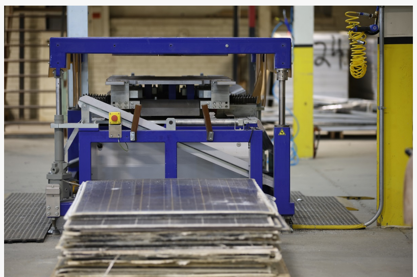
Commercial Solar Panel Recycling Deframer Phillipsburg 2024
