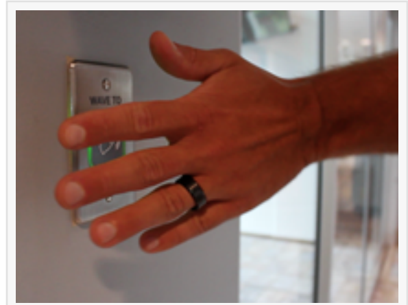
A hand sensor to automatically open the door
