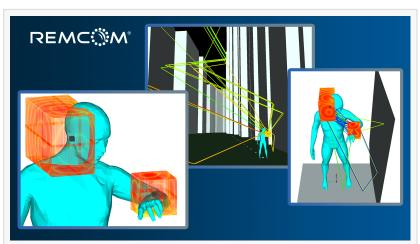
Remcom's Huygens surface capability enables the analysis of mobility, multipath, and interactions with body-worn devices in realistic environments.
