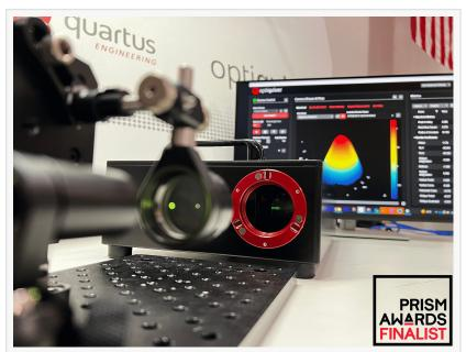
OptiQuiverTM 's versatility that combines the capabilities of many legacy tools ensures reliability in wavefront measurement, active lens alignment, bore sighting, and lens characterization.
