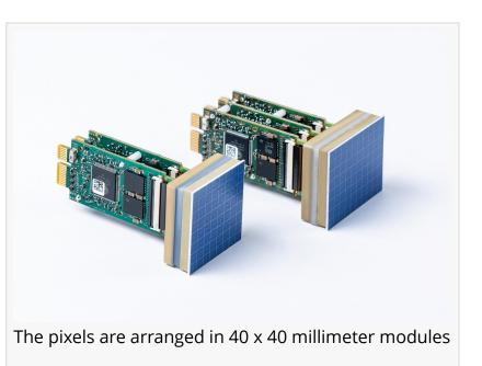
Watttron's cera2heat system can generate defined heterogeneous heating fields for problem areas using a large number of individually controllable small heating pixels. This allows the polymer film to be heated in a targeted manner and the flow behavior of the material to be optimally adapted to the desired packaging shape. This ensures a uniform wall thickness and
