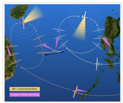
Diagram showing UAS Concept Of Operation for ISR and Communications using Power Beaming to extend operating capability
