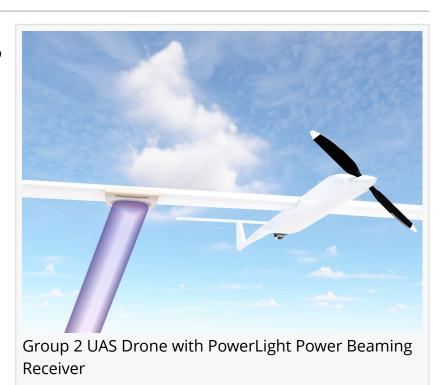
wireless power beaming to a Group-2 Unmanned Aerial System (UAS) aloft at 5,000 feet altitude, allowing it to rapidly recharge in flight and to conduct its mission without landing. The demonstration program, called Power TRansmitted Over Laser to UAS (PTROL-UAS), is part of the DOD's initiative to maximize effectiveness of autonomous systems by extending their range, operational endurance, and payload capacities to conduct critical surveillance and communications missions.
