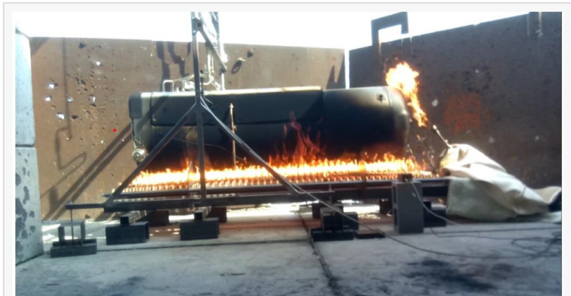
Liquid hydrogen storage solution for trucks by SAG Group during the Bonfire Test
