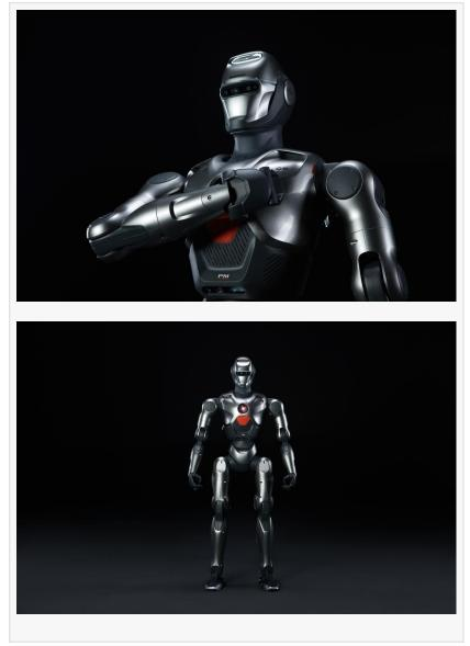
weighs approximately 40 kilograms, and features 24 degrees of freedom, achieving a movement speed of 2 meters per second. Its 320-degree waist rotation enables complex motions, complemented by mechanical and natural humanoid gait walking modes. Advanced optical motion capture technology and an end-to-end neural network solution allow the robot to accurately replicate human motion, making it highly adaptable to diverse environments.
