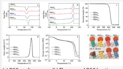
(a) DSC cooling scans; (b) The second DSC heating scans; (c) TGA curves; (d) DTG curves; (e) Storage modulus plots; (f) Digital photos showing heat resistance by observing deformation of the samples after maintaining at 150 °C for 30 min.
